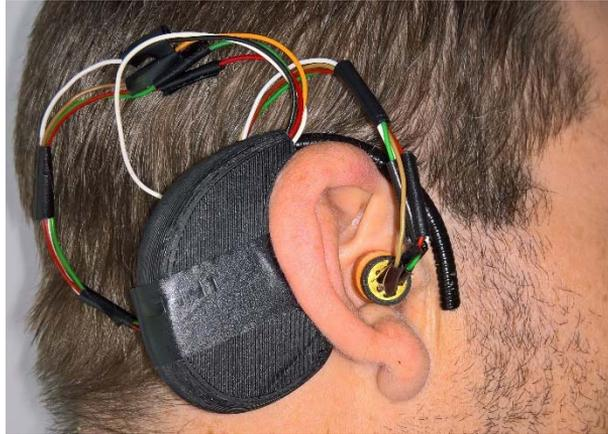
*Figure I.1 | The wearable ear thermometer CORTES<sup>2</sup>.*
