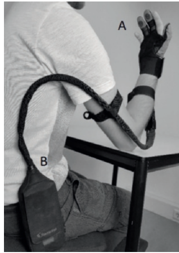
Figure 5.1 The ironHand system. A: Control unit, B: Glove.
