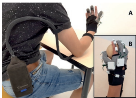
Figure 9.1 Representation of instrumentation of the experiment. A) shows the entire SEM Glove™ with pressure sensors placed on the grey circles, B) shows the SEM Glove with the white inertial measurement system.
