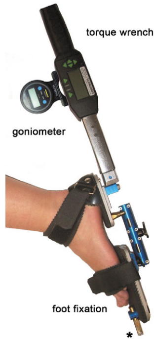
Figure 2.4: Photographic illustration of the hand held dynamometer
