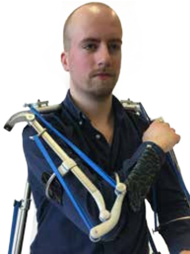
Figuur 5: prototype armondersteuner (Flexension A-Gear)
