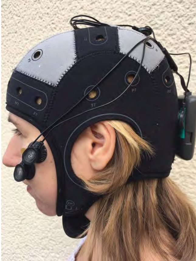
Figure 7.2 | Head cap with portable wireless tDCS stimulator.
