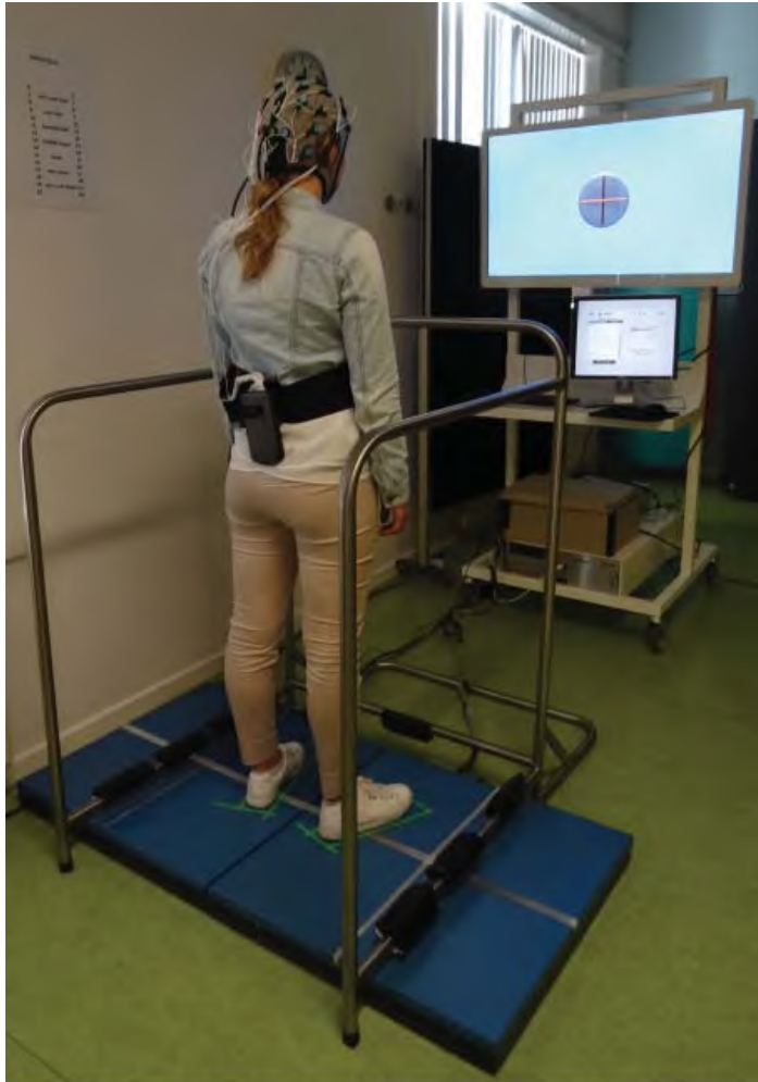
Figure 7.3 | Balance workstation with double force platforms, visual feedback and concurrent measured EEG.
