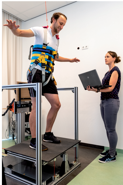
Figure 9.1. Balance board set-up. Springs were attached to each side of the front of the balance board. Rotational stiffness could be adjusted (0-220 Nm/rad) by using either one or two parallel springs on each side, by altering the springs' moment arm, or by changing the springs themselves (800 N/m vs. 390 N/m). Patients wore a safety harness.
